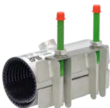
729/D2 (FST 20) Double band repair clamp, EPDM,ribs, stainless steel 304/316 with flanged outlet 10/16 bars
