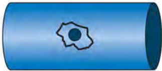
Damage caused by service crane or breaking-off of branching section
