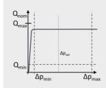
Deltaflow<sup>TM</sup> maintains a very precise +/-5% constant control  $\Delta p$  across the branch (p 1 – p 2). The total flow of the modulating control valves is kept stable at whichever setpoint (Q) regardless of outside influences.
