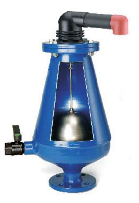
AVK combination air valves combine an air & vacuum orifice and an automatic air release orifice in a single body. The innovative design with a large air gap between liquid and sealing system ensures a reliable function even when used with aggressive liquids and liquids with solid particles.
