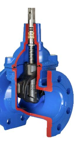
The wedge is the heart of a gate valve and the quality of the wedge rubber is crucial for the valve function and durability. AVK wedges are fully vulcanised with AVK's rubber compound with outstanding characteristics. The double bonding vulcanisation process ensures maximum adhesion of the rubber and prevents creeping corrosion.
