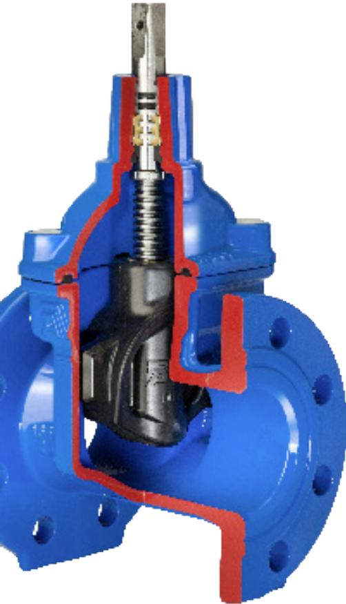
The wedge is the heart of a gate valve and the quality of the wedge rubber is crucial for the valve function and durability. AVK wedges are fully vulcanised with AVK's rubber compound with outstanding characteristics. The double bonding vulcanisation process ensures maximum adhesion of the rubber and prevents creeping corrosion.
