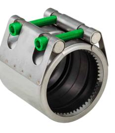
AVK's range of Repico® couplings in stainless steel 316 comprises tensile "Grip" couplings for all metal pipe materials up to DN400, and non-tensile "Slip" couplings for all pipe materials up to DN2000. Repico® couplings are suitable for water and wastewater applications.
