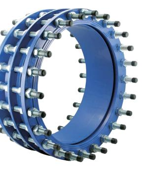
AVK dismantling joints provide easy installation and disassembly of flanged pipework and equipment and compensate for axial displacement of the pipe during installation and dismantling. The range is available in DN40-2600 in PN10/16 and up to DN1200 in PN25.
