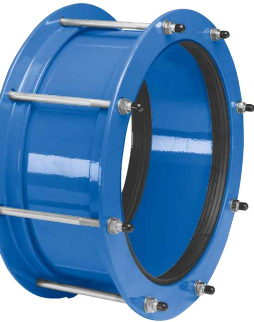
AVK's range of fabricated fittings comprises non-tensile straight couplings, step couplings and flange adaptors in DN350-2000. The range is suitable for ductile and grey cast iron, steel, uPVC and GRP pipes for water and wastewater applications up to 25 bar.
