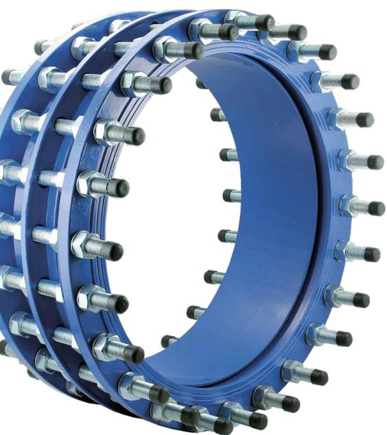
AVK dismantling joints provide easy installation and disassembly of flanged pipework and equipment and compensate for axial displacement of the pipe during installation and dismantling. The range is available in DN40-2600 in PN10/16 and up to DN1200 in PN25.
