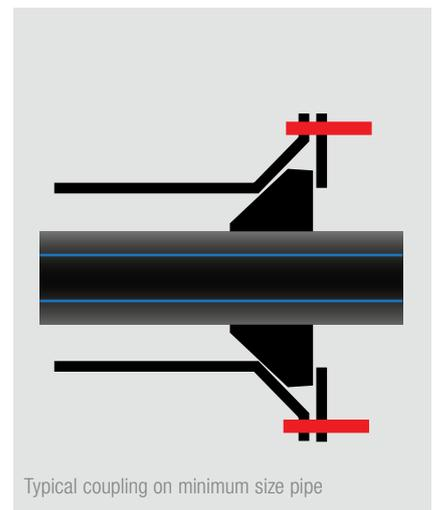
Typical coupling on minimum size pipe
