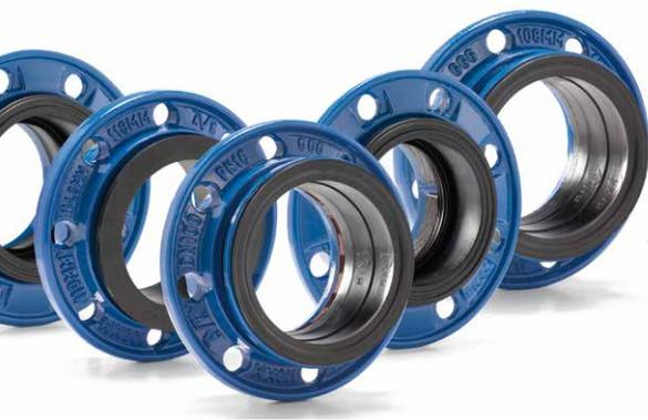
AVK's combi-flange system comprises tensile combi-flanges for PE, PVC and ductile iron pipes in DN50-300 as well as non-tensile combi-flanges for PVC, ductile iron and steel pipes in DN50-600. The combi-flanges are suitable for water and wastewater applications.
