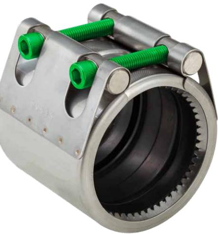
AVK's range of Repico® couplings in stainless steel 316 comprises tensile "Grip" couplings for all metal pipe materials up to DN400, and non-tensile "Slip" couplings for all pipe materials up to DN2000. Repico® couplings are suitable for water and wastewater applications.
